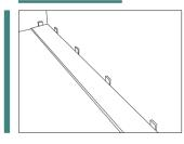
4• Place wedges around the sides to create an expansion gap.
