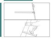
5• Cut the last row of strips to the required length, again allowing for an expansion gap. Use a metal pull bar to ensure the strips are flat.
