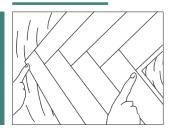
1. The subfloor must be flat and dry. In the case of panel, herringbone and mitred herringbone patterns, start fitting from the central axis of the room. For strip flooring, begin laying in a corner with the tongue against the wall.
